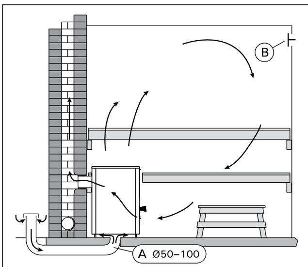
Figure 4. Gravity exhaust ventilation
