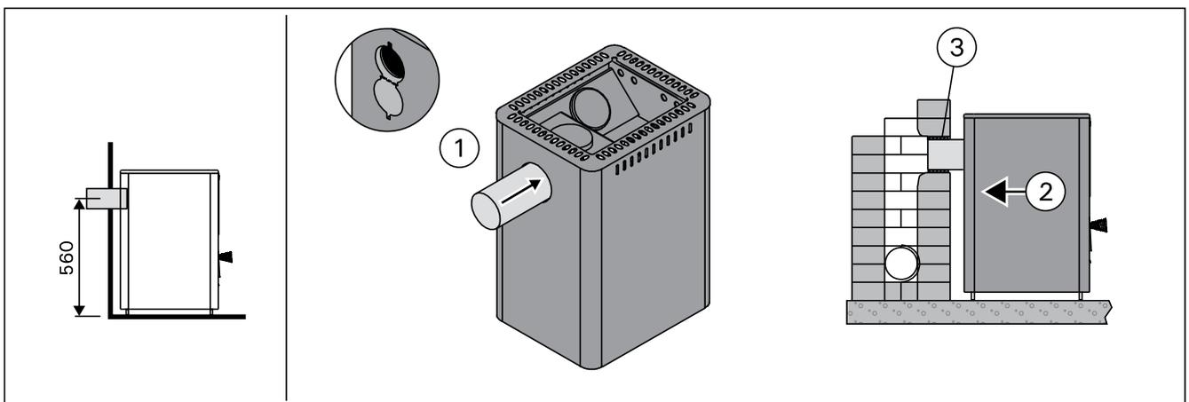
Figure 9. Connecting the stove to a masonry flue via the rear connection opening (all dimensions in millimeters)
