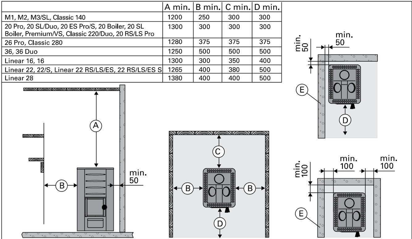
Figure 7. Safety distances (all dimensions in millimeters)
