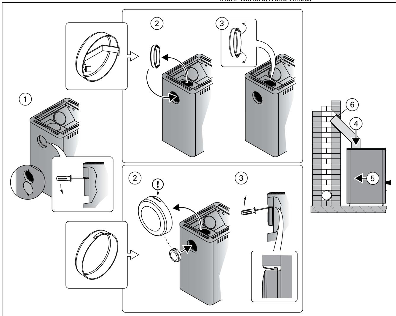
Figure 10. Connecting the stove to a masonry flue via the upper connection opening (all dimensions in millimeters)
