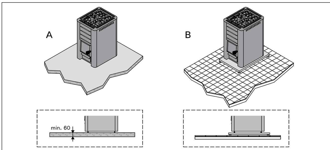
Figure 6. Protecting the floor (all dimensions in millimeters)
