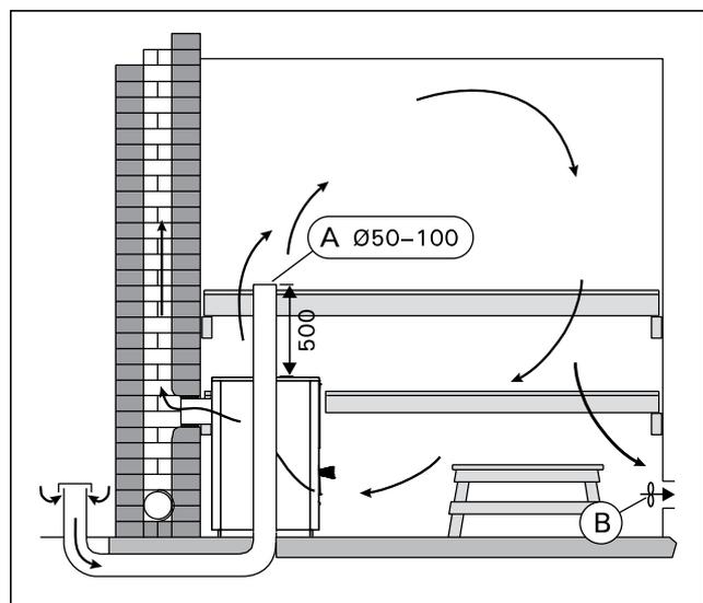
Figure 5. Mechanical exhaust ventilation
