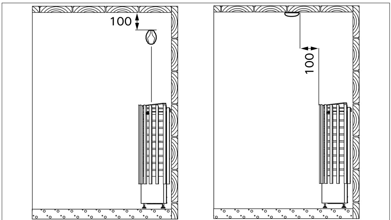
Figure 8. Installing the sensor (all dimensions in millimeters)
