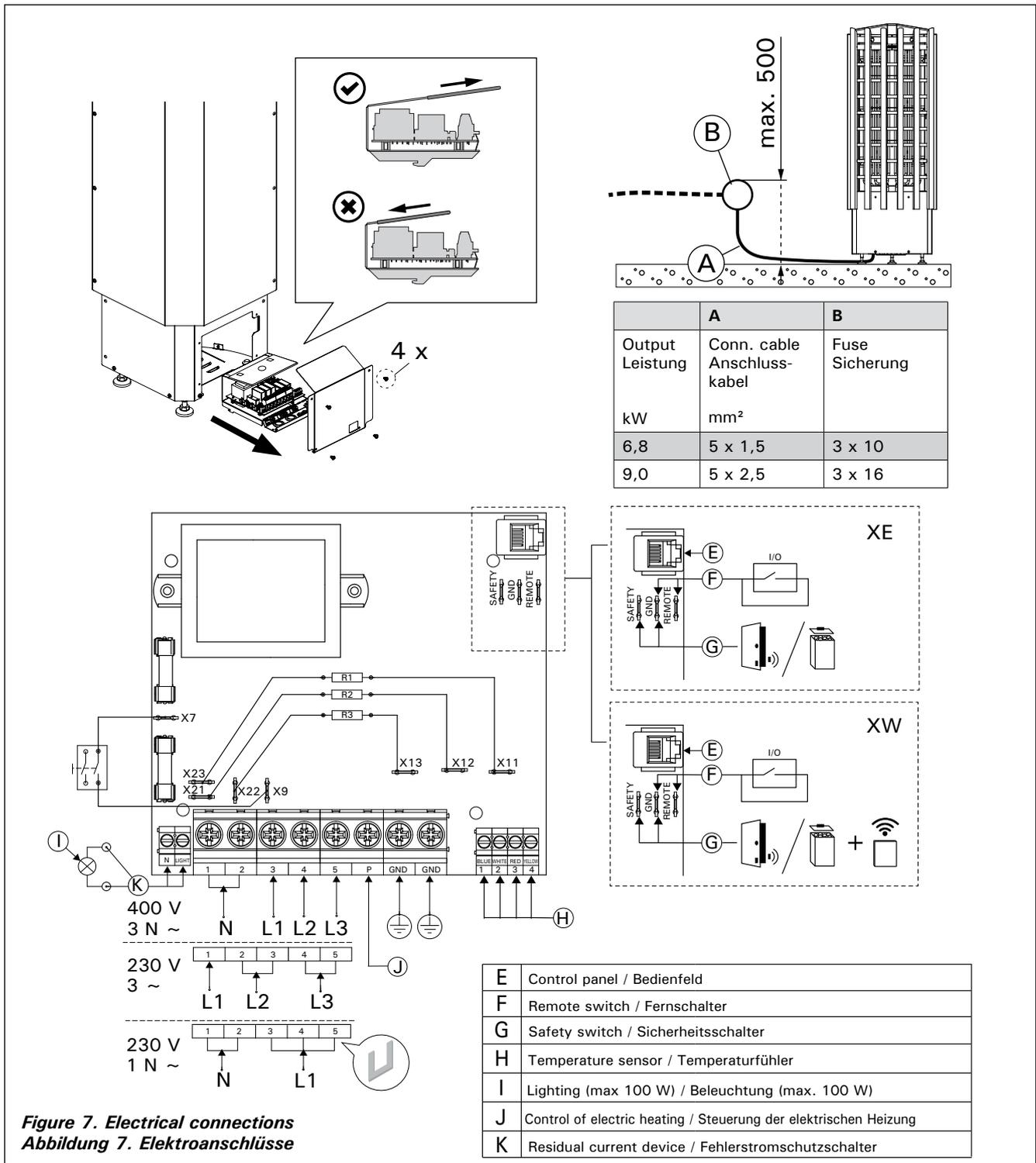
**Figure 7. Electrical connections**
