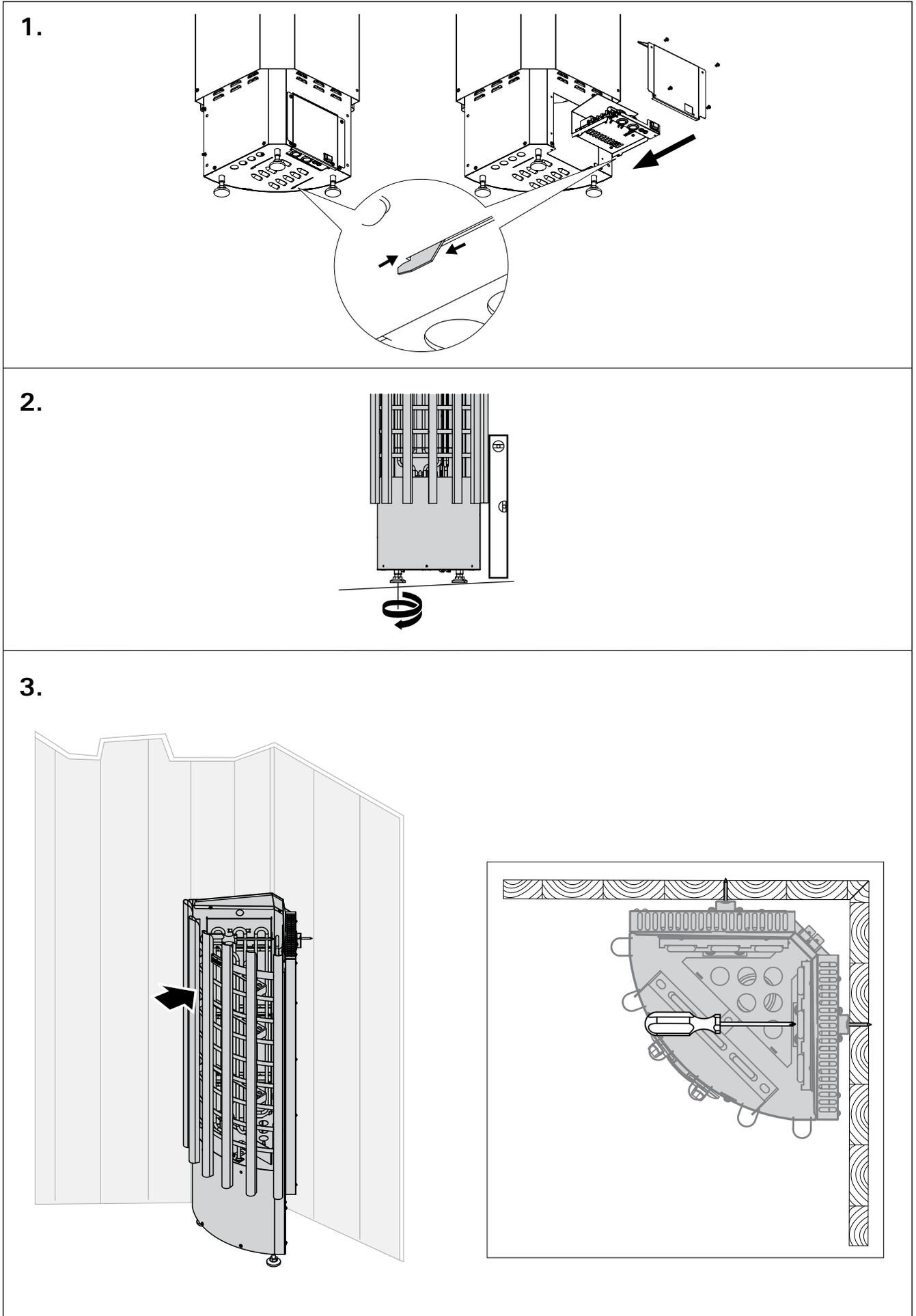
Figure 10. Installing the heater
