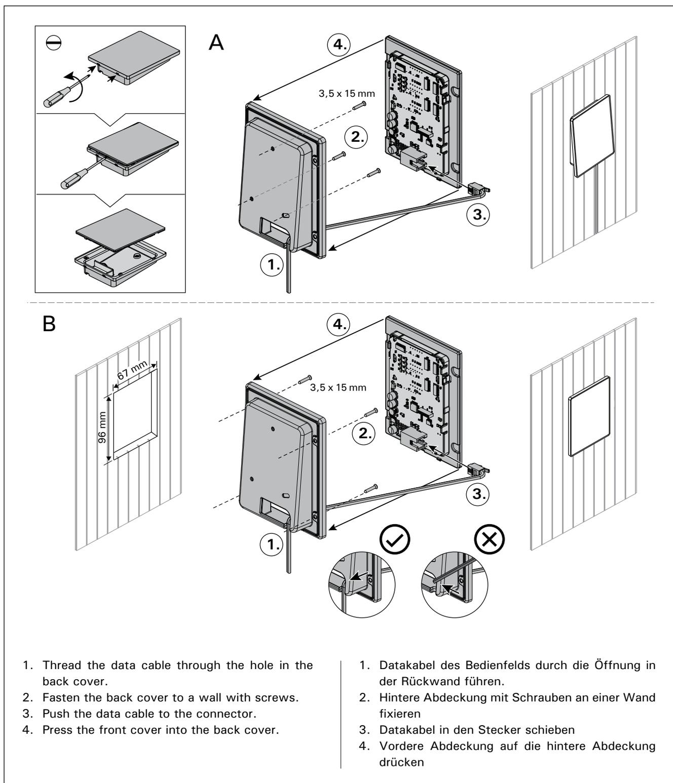
Figure 9. Installing the control panel (all dimensions in millimeters)
